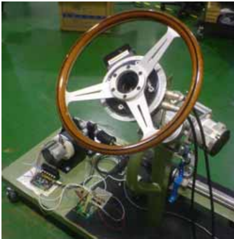
Fig. 14. Steering wheel sensor for measuring steering torque and angle.
