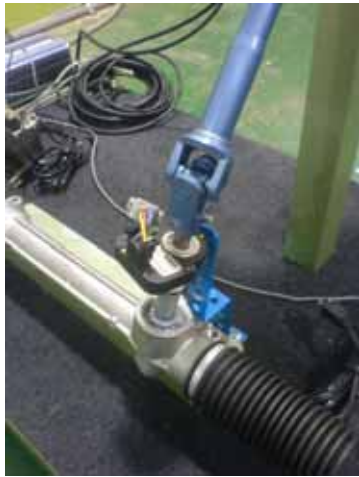
Fig. 8. Steering wheel angle sensor for the force feedback control system.
