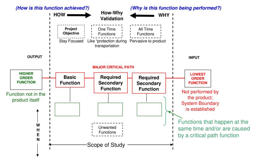
Three types of Secondary Functions: Required, aesthetic (housing, packaging, color, etc.), and unwanted (noise, vibration, etc.).
