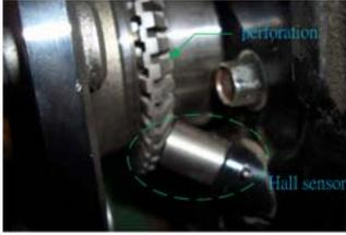
Figure 5. Wheel speed detection.
