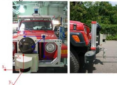
Figure 6. LiDAR and camera coordinate systems.
