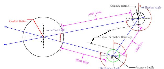
Fig.2. Geometry model of two conflicting objects
